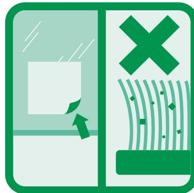
Do not use a razor blade, wire wool or any other metal item to remove stubborn marks. These will leave metal particles on the coating that appear as scratches. Where this occurs inadvertently, these marks may be removed using weak solutions of acids. However, this should be regarded as an extraordinary remedial action, requiring particular advice and taking account of any health and safety issues.
